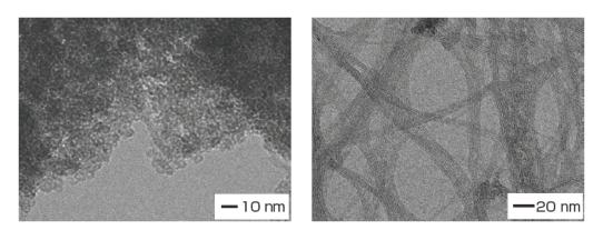
Fig. 4 TEM photographs of allophane and imogolite (Left: allophane<sup>[7]</sup>, right: imogolite<sup>[7]</sup>)
