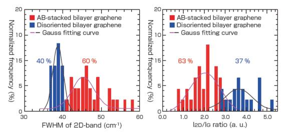
**Fig. 11 The histograms of FWHM values of 2D-band and intensity ration of 2D-band/G-band**<sup>[14]</sup> Red bar is AB-stacked bilayer graphene and blue bar is disorder-stacked bilayer graphene. Copyright (2014), with permission from Elsevier
