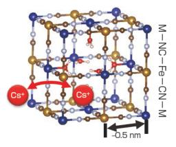
Fig. 1 The crystal structure of hexacyanoferrate  $A_yM[Fe(CN)_6]_{1-x} \cdot zH_2O$ , where A and M indicate the cations and the transition metal ions of Fe, Cu, Co, or others The red atoms around the vacancy show the oxygen in the H<sub>2</sub>O molecule.
