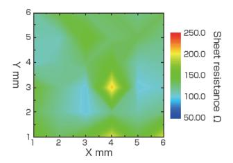
Fig. 13 The sheet resistance map of graphene after wet doping with gold chloride<sup>[14]</sup> Copyright (2014), with permission from Elsevier
