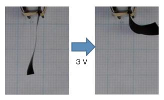
Fig. 5 Deformation of the bucky gel actuator at 3 V applied voltage
