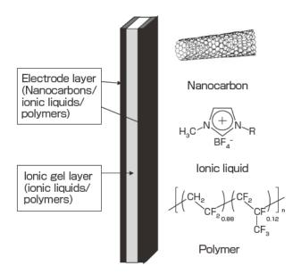
Fig. 3 Schematic diagram of the structure of the bucky gel actuator
