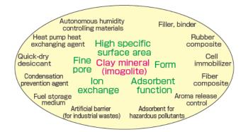
Fig. 5 Fields in which imogolite is used
