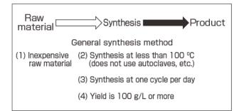
Fig. 7 Conditions necessary for the synthesis of new adsorbents
