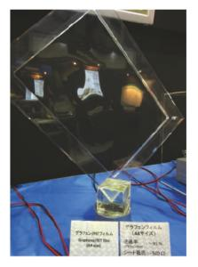
Fig. 14 A4 size large area graphene transparent conductive film
