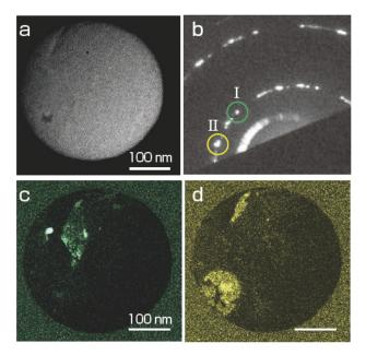
Fig. 16 (a) TEM image, (b) the selected area electron diffraction pattern, and (c) (d) The dark-field TEM images<sup>[15]</sup> Copyright (2015), with permission from Elsevier
