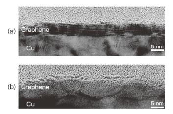
Fig. 7 Cross-sectional TEM images of synthesized graphene by surface-wave plasma using (a) the He/H<sub>2</sub>/CH<sub>4</sub> gas mixture and (b) the Ar/H<sub>2</sub>/CH<sub>4</sub> gas mixture<sup>[13]</sup> Copyright (2014) The Japan Society of Applied Physics
