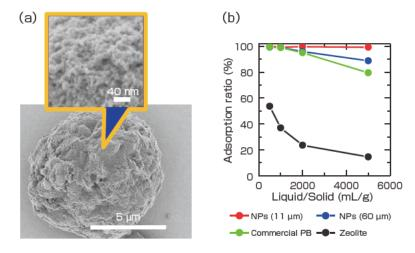
Fig. 5 (a) Electron microscope image of PB nanoparticle powder. (b) Liquid–solid ratio dependency of adsorption performance when various cesium adsorbents are added to the water after washing the incinerated ash<sup>[3][30]</sup>
