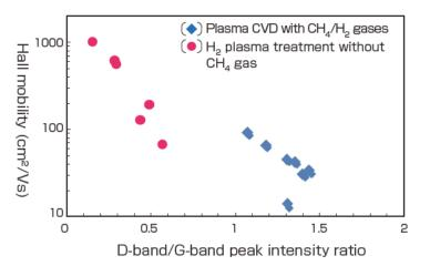
Fig. 15 The relationship between the Hall mobility and Raman intensity D-band/G-band ratio<sup>[15]</sup>
