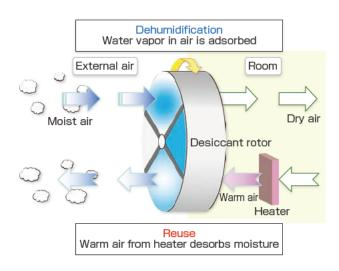
Fig. 1 Outline of the desiccant air conditioner that uses water vapor adsorbent
