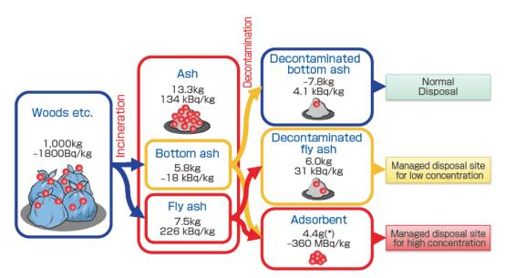
Fig. 8 Example of volume reduction when the incinerated ash processing technology is used<sup>[6]</sup>
