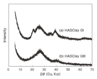
Fig. 8 Powder x-ray diffraction pattern of HASClay
