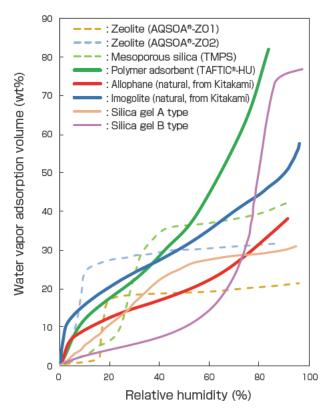
Fig. 2 Water vapor adsorption isothermal curve of the adsorbents that can be reused by low-temperature treatment (AQSOA\*-Z01<sup>[2]</sup>, AQSOA\*-Z02<sup>[2]</sup>, TMPS<sup>[3]</sup>, TAFTIC\*-HU<sup>[4]</sup>)
