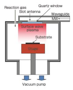
Fig. 1 Schematic illustration of the surface-wave microwave plasma CVD equipment<sup>[13]</sup> Copyright (2014) The Japan Society of Applied Physics
