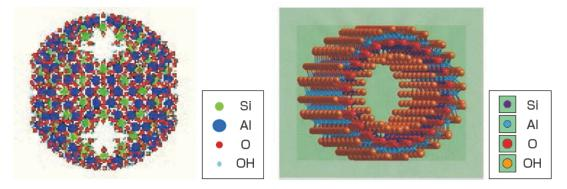
Fig. 3 Structural models of allophane and imogolite (Left: allophane<sup>[5]</sup>, right: imogolite<sup>[6]</sup>)
