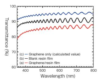
Fig. 12 Optical transmittance of base resin film and graphene/resin films  $\ensuremath{^{[4]}}$
