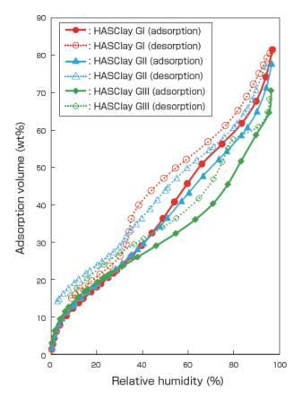
Fig. 11 Water vapor adsorption isothermal curves of HASClay
