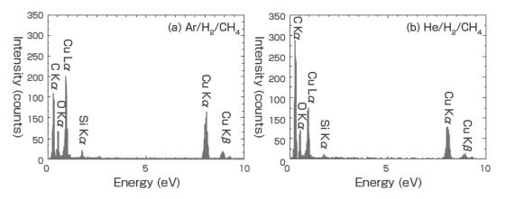
Fig. 6 EDX spectrum of Monolayer and/or bilayer graphene synthesized using (a) the Ar/H<sub>2</sub>/CH<sub>4</sub> gas mixture and (b) the He/H<sub>2</sub>/CH<sub>4</sub> gas mixture<sup>[13]</sup> Copyright (2014) The Japan Society of Applied Physics
