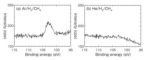
Fig. 5 XPS spectrum of Si 2*p* binding energy for synthesized graphene using (a) the Ar/H<sub>2</sub>/ CH<sub>4</sub> gas mixture and (b) the He/H<sub>2</sub>/CH<sub>4</sub> gas mixture<sup>[13]</sup> Copyright (2014) The Japan Society of Applied Physics
