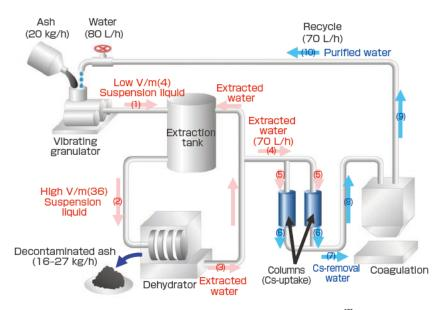
Fig. 7 Schematic view of the ash washing and recovery plant<sup>[6]</sup>
