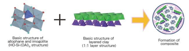
Fig. 6 Schematic diagram of the formation of new adsorbent structure
