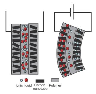
Fig. 4 Deformation response principle of the bucky gel actuator
