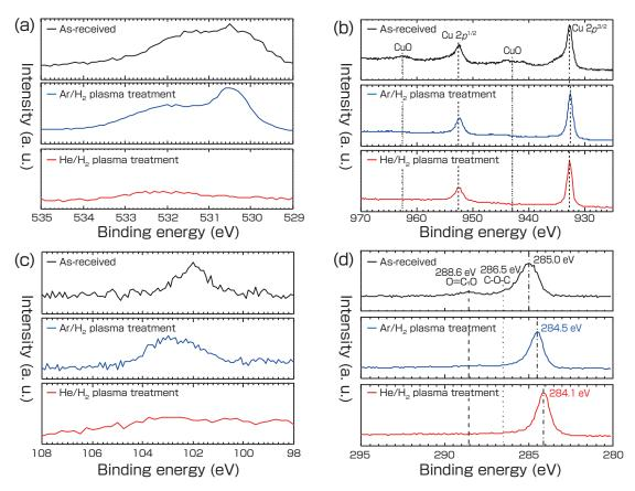
**Fig. 3 XPS spectrum of the copper foil with plasma pretreatment and without plasma pretreatment**<sup>[13]</sup> (a) O 1s binding energy, (b) Cu 2p binding energy, (c) Si 2p binding energy, (d) C 1s binding energy Copyright (2014) The Japan Society of Applied Physics
