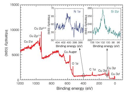
**Fig. 2 XPS survey spectrum of the as-received copper foil**<sup>[13]</sup> Copyright (2014) The Japan Society of Applied Physics
