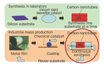
Fig. 6 Lab-scale vs. mass production process
