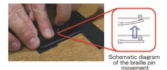
Fig. 6 Braille display using the bucky gel actuator
