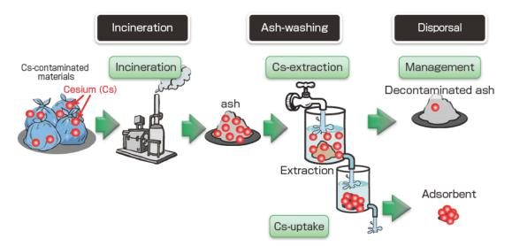
Fig. 3 Outline of volume reduction of vegetal contaminants and incinerated ash using PB nanoparticles<sup>[6]</sup>
