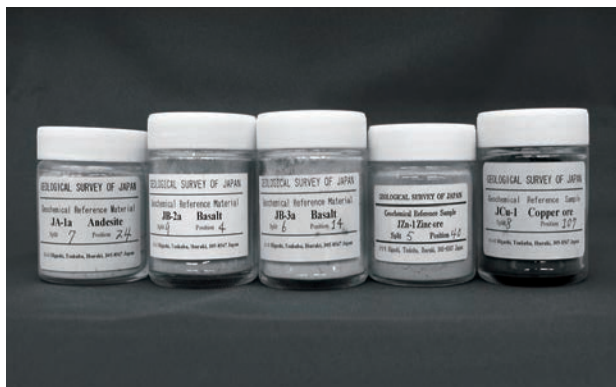
Fig. 1 Geochemical reference materials published by GSJ From left: JA-1a, JB-2a, JB-3a, JZn-1, and JCu-1 Powdered samples are packed in bottles and distributed.
