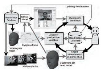
Fig. 5 A system to produce eyeglass frames according to the "Finding well-fitting products" approach (From M. Mochimaru et al., Synthesiology, Vol.1, No.1 [7])
