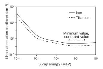
Fig. 2 Linear attenuation coefficients of iron and titanium at 10 keV ~ 100  $\text{MeV}^{[6]}$
