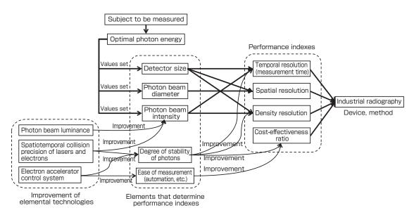
Fig. 8 Improvement of elemental technologies, elements that determine the performance index, and relationship of the sophistication of devices and methods
