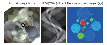
**Fig. 6 (Left) Sample photograph, (center) sinogram, and (right) CT image**<sup>[9]</sup> The samples include water in a beaker and rods of various metals such as silicon, aluminum, and tungsten. Blue to green represent the low density ranges, while yellow to red show the high density ranges.
