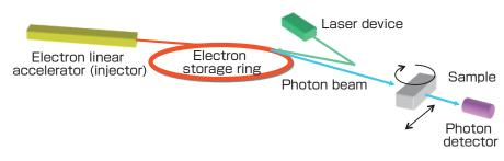
Fig. 4 LCS photon CT system using the electron accelerator
