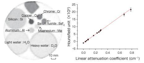
Fig. 7 (Left) Plot of the linear attenuation coefficients of various materials and the CT values expressed by HU.<sup>[10]</sup> The symbols in the diagram represent the substances, e.g.  $D_2O$  = heavy water.
