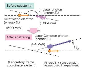
Fig. 1 Kinematics of laser Compton scattering
