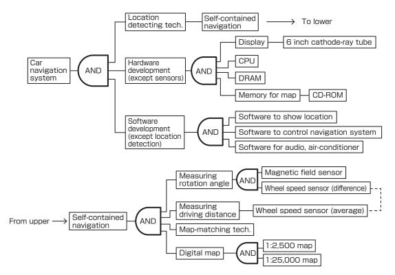
Fig. 10 Technology architecture when the first car navigation system was finished (1989 model)
