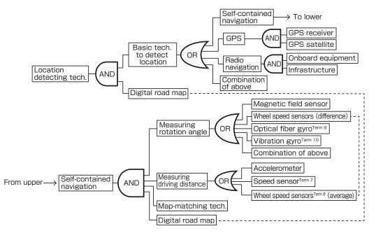
Fig. 7 R&D issues for detecting current location of car navigation systems (Technology architecture)
