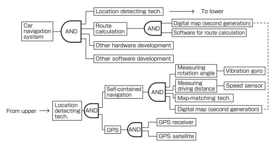
Fig. 12 Technology architecture of 1992 model (second generation)
