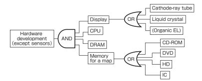
Fig. 8 Element technologies for hardware development
