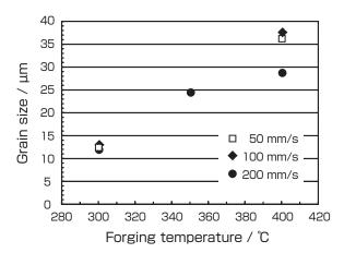
Fig. 4 Variation in grain size as a function of the processing temperature for AZ91 (Mg-9 mass% Al-1 mass% Zn) magnesium alloy continuous cast bar (reduction ratio : 40 %)
