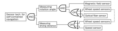
Fig. 11 Change of sensors from 1989 model to 1991 model
