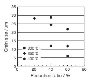
Fig. 3 Variation in grain size as a function of the reduction ratio for AZ91 (Mg-9 mass% Al-1 mass% Zn) magnesium alloy continuous cast bar (deformation speed: 200 mm/s)
