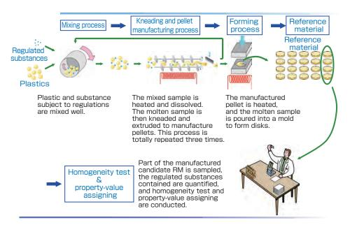
Fig. 3 Manufacturing process of plastic RMs (example)
