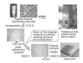
Fig. 8 Outline of the developed low-temperature forging process
