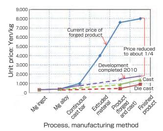
Fig. 1 Cost estimate of the magnesium alloy parts
