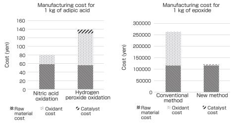
Fig. 9 Comparison of the manufacturing cost
