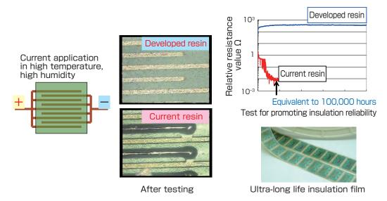
Fig. 12 Performance evaluation of the fabricated insulation material
