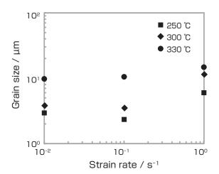
Fig. 2 Grain size of AZ91 (Mg-9 mass% Al-1 mass% Zn) magnesium alloy continuous cast bar after high-temperature compression (reduction ratio : 80 %)
