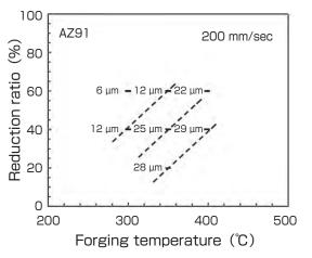
Reference: Relationship between the forging temperature, reduction ratio, and grain diameter created from the experimental result
