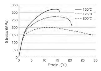
Fig. 10 Result of the compression test of AZX91 + 0.2 mass% Ca alloy that underwent grain refinement
