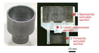
Fig. 7 Example of the forged prototype (Material: AZ91 magnesium alloy continuous cast bar)
