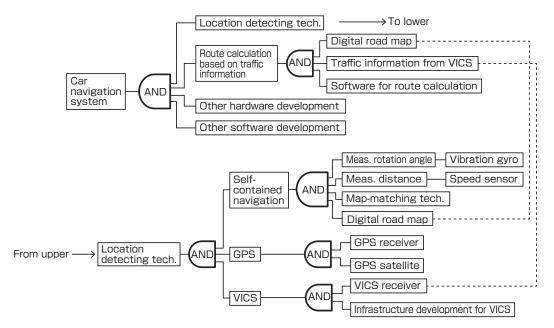
Fig. 13 Technology architecture of the third generation of car navigation systems
