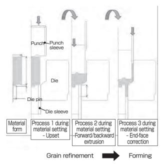
Fig. 6 Forging process using the servo press
