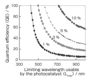
Fig. 8 Quantum efficiency (QE) of the iron ion redox reaction of photocatalyst (E<sup>°</sup> = +0.77 V) and the theoretically limiting solar energy conversion efficiency  $(\eta_{sun}^{m})$
