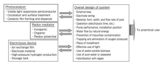
Fig. 6 Elemental technology development and scenario for achieving practical use of the photocatalysis-electrolysis hybrid system
