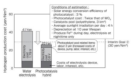
Fig. 9 Detailed cost estimation of the photocatalysis-electrolysis hybrid system
