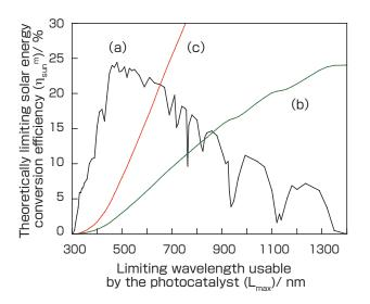
Fig. 7 Theoretically limiting solar energy conversion efficiency ( $\eta_{sun}^{m}$ ) for the redox reaction of photocatalyst In the case where the quantum efficiency and photoabsorption efficiency up to the limiting wavelength that can be used by photocatalyst is 100 %; (a) Sunlight spectrum, (b) iron ion redox reaction, and (c)  $E^{\circ} = 0$  redox reaction.
