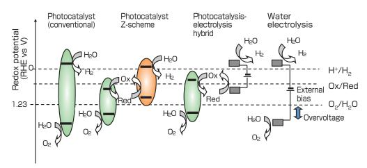
**Fig. 4 Various hydrogen production technologies from water and their potential map** Ox and Red are the oxidants and reductants of the redox mediator.
