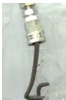
Fig. 5 Dewatered sludge supply by high-pressure sludge pump
