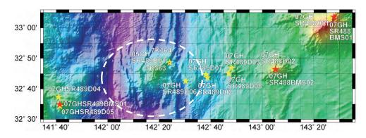
**Fig. 3 Sampling of basement rock in the offshore region of East Japan (original map from Ishizuka)** Sampling points (red star – boring, yellow star – dredging) in the area around Mogi Seamount (surrounded by white dashed line) off the coast of Hachijo Shima Island
