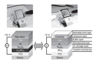
Fig. 4 Photograph and structure of the all-solid-state electrochromic switchable mirror device
