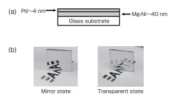
Fig. 1 (a) Basic structure of the switchable mirror, and (b) the magnesium-nickel (Pd/Mg\_ $\beta$ Ni) switchable mirror thin film with excellent optical property developed at AIST
