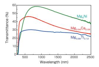
Fig. 2 Comparison of the transmission spectra in the transparent state of the magnesium-nickel ( $Mg_6Ni$ ) switchable mirror, magnesium-titanium ( $Mg_{0.88}Ti_{0.12}$ ) switchable mirror, and magnesium-calcium ( $Mg_{0.94}Ca_{0.06}$ ) switchable mirror
