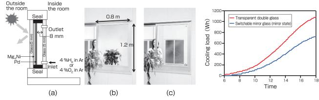
**Fig. 7 Switchable mirror windowpane of actual size** (a) Structure, (b) mirror state, and (c) transparent state
