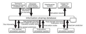
Fig. 9 System configuration for Toyohashi City demonstration experiment
