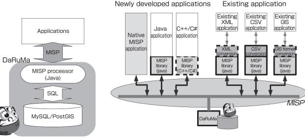
Fig. 6 System linkage by mitigation information sharing protocol (MISP) and DaRuMa
