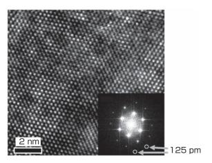
Fig. 10 Performance examination of the second low-voltage microscope (TEM)
