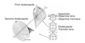
Fig. 5 Construction and calculated electron-beam trajectory of new chromatic aberration corrector
