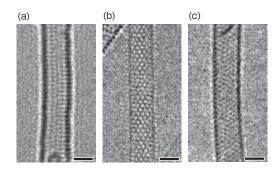
**Fig. 1 Comparison of TEM images of SWCNTs**(a) Recorded at an acceleration voltage of 120 kV without spherical aberration (Cs) correction, (b) recorded at 120 kV with Cs correction, (c) recorded at 80 kV with Cs correction Scale bar = 1 nm
