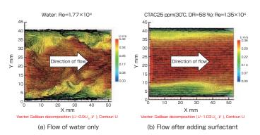
Fig. 2 Changes in flow due to micelle network
