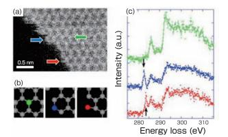
Fig. 12 Observation of electronic states with low-voltage STEM-EELS
