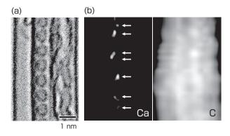
**Fig. 11 Elemental analysis with low-voltage STEM-EELS** (a) ADF-STEM image, (b) elemental maps for calcium and carbon (left and right, respectively)
