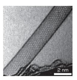
Fig. 9 TEM image of a SWCNT recorded at an acceleration voltage of 30  $\mbox{kV}$
