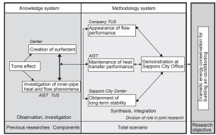
Fig. 3 Scenario for energy savings using surfactant in air conditioning of buildings
