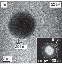
Fig. 8 Performance examination of the first low-voltage microscope in TEM mode
