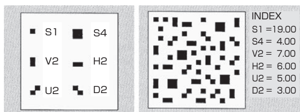
Fig. 9 Simultaneous recognition (/enumeration) of multiple objects [5][6]
