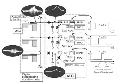
Fig. 5 Digital piezoelectric accelerometer
