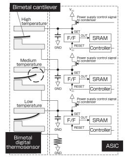
Fig. 4 Digital bimetal thermosensor
