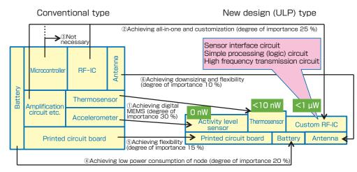
Fig. 6 Comparison of the ULP wireless sensor and the conventional sensor
