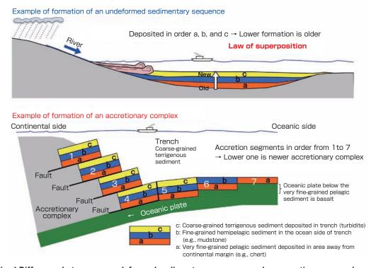
Fig. 4 Difference between an undeformed sedimentary sequence and an accretionary complex.
