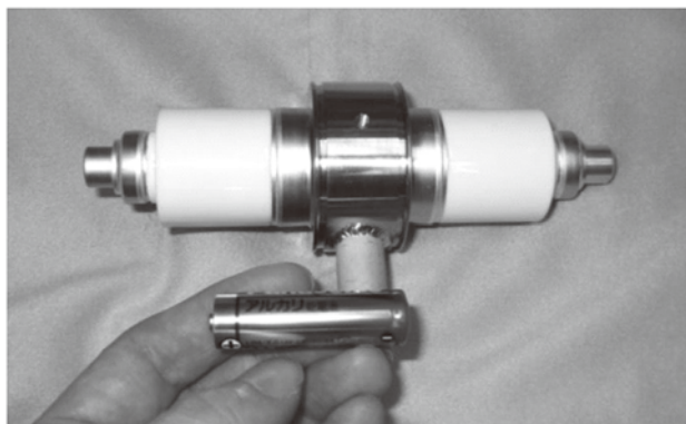
Fig. 1 X-ray tube using the carbon nanostructure electron source.
