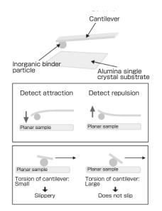
Fig. 6 Measurement of inter-surface interactive force.
