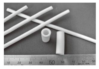
Fig. 5 Alumina ceramics fabricated using inorganic binder technology.
