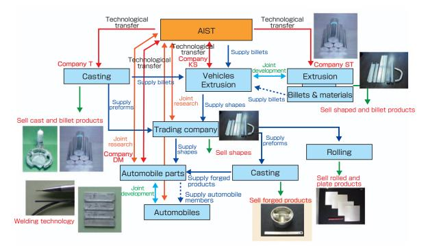
Fig. 9 Mass production system for noncombustible magnesium alloy.
