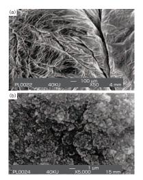
Fig. 2 Surface structure of oxide film in pure magnesium.
