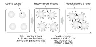
Fig. 4 Fixing of organic molecule and application of reaction trigger to reduce the amount of organic binder.
