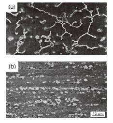
Fig. 5 Structure of noncombustible magnesium alloy (AMX602). a: Solidified structure, b: Structure after extrusion.
