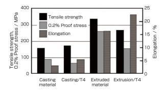
Fig. 6 Mechanical property of noncombustible magnesium alloy (AMX602).
