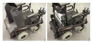
Fig. 12 Mounted PC. Right photo shows the device exposed without the cover. The PC is mounted behind the seat.
