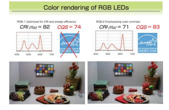
Fig. 3 Color rendering of RGB LEDs.
