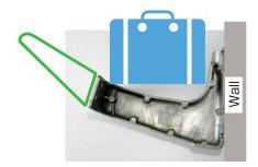
Fig. 11 Luggage shelf support made of noncombustible magnesium alloy (AZX912).
