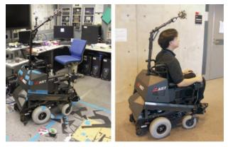
**Fig. 13 Consideration of the exterior design.** Left photo shows the process of designing. The design was determined after repeated trials. The right photo is the design for Prototype 1. This model was used for the press release.
