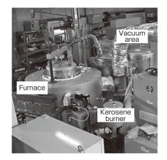
Fig. 4 Smelting furnace for noncombustible magnesium alloy equipped with reduced pressure refinement mechanism (capacity100 kg).
