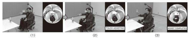
Fig. 17 Automatic assistance is provided to the position that allows the hand to reach the bottle, by recognizing the rider's gesture.
