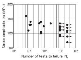
Fig. 7 Endurance strength assessment of noncombustible magnesium alloy (AMX602).
