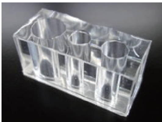
Fig. 3 Photograph of device for sorting motile spermatozoa
