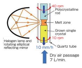
Fig. 6 Growth condition of garnet-type lithium solid electrolyte
