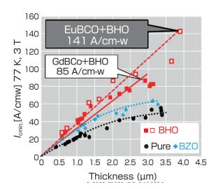
Fig. 10 Effect of artificial pinning center material against film thickness dependency of in-field  $I_c$  property for PLD film<sup>[31]</sup>
