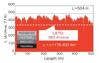
Fig. 6 Long-length tape in IBAD-PLD tape material<sup>[18]</sup>
