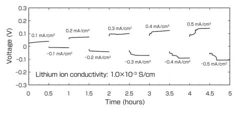
Fig. 10 Result of internal short-circuit test
