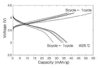
Fig. 14 Charge/discharge property of Li / garnet-type lithium solid electrolyte / NCA all-solid-state lithium secondary battery at 25 °C
