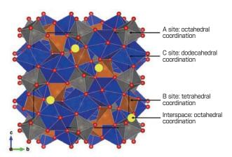
Fig. 3 Crystal structure of garnet-type lithium solid electrolyte
