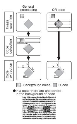
Fig. 3 Detection processes of position and shape of code
