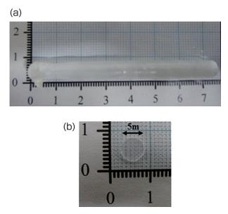
Fig. 7 (a) Grown single crystal of garnet-type lithium solid electrolyte Li<sub>6.5</sub>La<sub>3</sub>Zr<sub>1.5</sub>Nb<sub>0.5</sub>O<sub>12</sub>; (b) cut and polished single crystal plate
