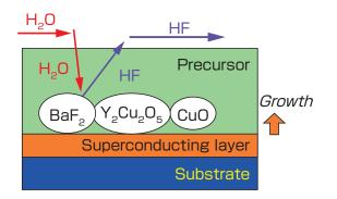
Fig. 7 Conceptual diagram showing reaction in TFA-MOD method
