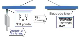
Fig. 11 Schematic diagram of NCA electrode film forming onto garnet-type lithium solid electrolyte single crystal substrate using the AD method
