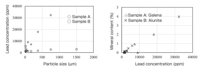
Fig. 3 Relationships among lead concentration, particle size, and mineral content in naturally occurring contaminated soil samples
