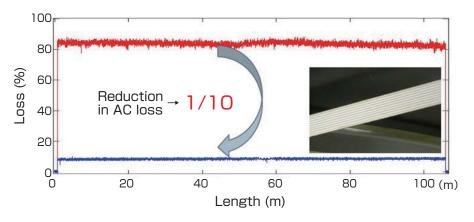
Fig. 13 Achievement of low AC loss in 100 m class tape material using scribing technology  $^{\!\
