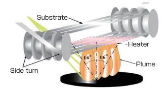
Fig. 5 Conceptual diagram of multi-plume and multiturn PLD system
