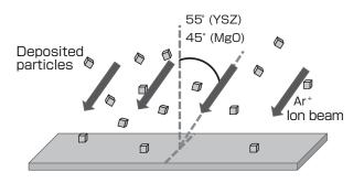
Fig. 3 Conceptual diagram of IBAD method
