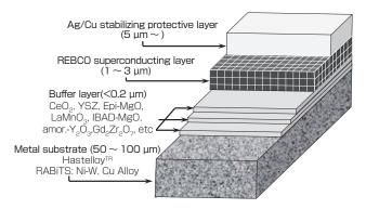
Fig. 2 Schematic diagram of REBCO tape structure
