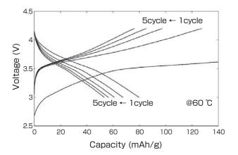
Fig. 13 Charge/discharge property of Li / garnet-type lithium solid electrolyte / NCA all-solid-state lithium secondary battery at 60 °C
