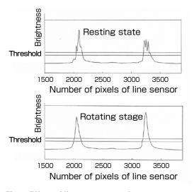
Fig. 3 Effect of line sensor rotation
