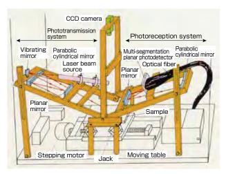
Fig. 4 Measurement system for curved mirror objects
