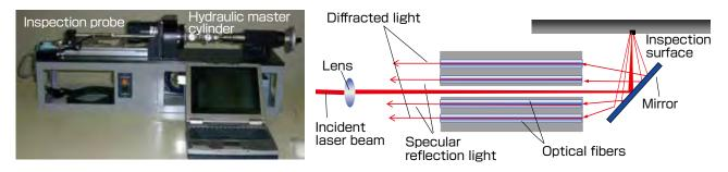
Fig. 8 Inspection system for inner wall surfaces of machined holes
