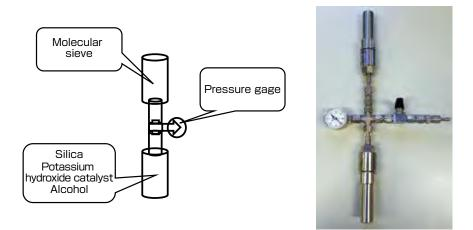
Fig. 6 Schematic diagram of reaction vessel for tetraalkoxylsilane and its  $\mathsf{photograph}^{^{[3]}}$
