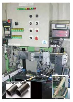
Fig. 10 Inspection system for outer surface flaws of cylindrical automobile parts
