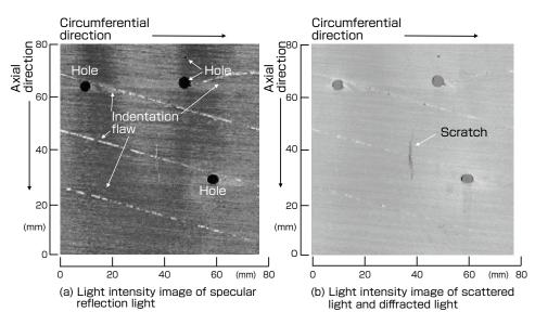
Fig. 9 Examples of inspection images of inner wall surfaces of machined holes
