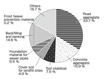
Fig. 3 Current situation of use of molten slag (from garbage and sewage sludge)^{\ensuremath{\text{I}}^2}
