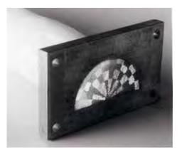
Fig. 6 Multi-segmentation planar photodetector
