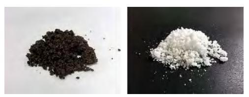
Fig. 7 Raw material molten slag (left) and synthesized silica with high specific surface area (right)
