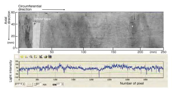
Fig. 12 Light intensity detection image of specular reflection light
