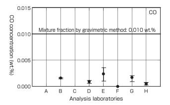
Fig. 11 Analysis result of carbon monoxide (CO) in the round-robin test<sup>[9]</sup>\*
