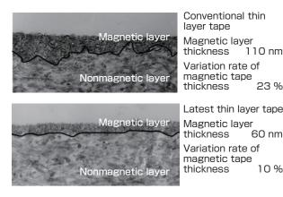
Fig. 10 TEM image of the tape cross-section
