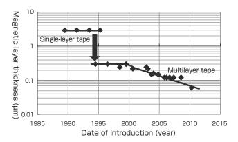
Fig. 4 Transition of the magnetic layer thickness<sup>[8][9]</sup>
