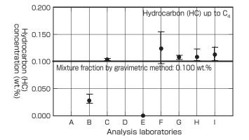
Fig. 9 Analysis result of hydrocarbon (HC) of C<sub>4</sub> or less in the round-robin test<sup>[9]</sup>\* \*Graph based on data of ref. [9]
