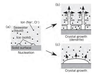
Fig. 2 Schematic of ice generation from seawater. Nucleation and growth of ice on a cooling solid surface.
