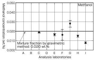
Fig. 10 Analysis result of methanol in the round-robin test<sup>[9]\*</sup> \*Graph based on data of ref. [9]
