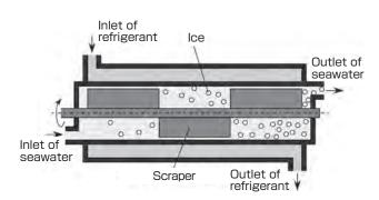
Fig. 3 Double-tube heat exchanger (generator) producing slurry ice from sea water
