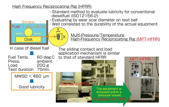
Fig. 6 Lubricity evaluation device and evaluation method
