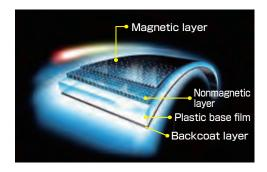
Fig. 2 Structure of the magnetic tape
