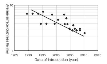
Fig. 5 Transition of the surface smoothness of tape
