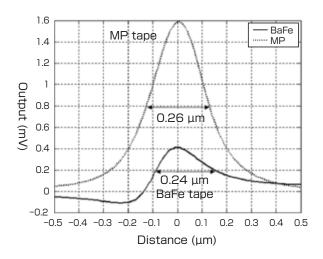
Fig. 8 Comparison of the isolated transition response of BaFe/MP
