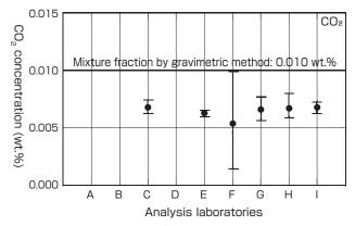
Fig. 12 Analysis result of carbon dioxide (CO<sub>2</sub>) in the round-robin test<sup>[9]\*</sup> \*Graph based on data of ref. [9]
