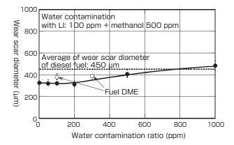
Fig. 8 Effect of water contamination on abrasion scar diameter<sup>[1]\*</sup> (water 0–1,000 ppm, methanol 500 ppm) \*Data added to ref. [1]
