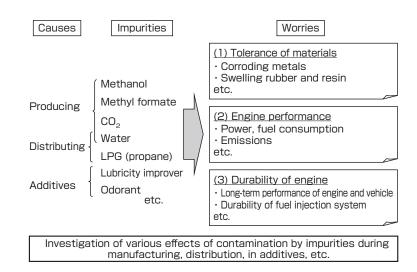
Fig. 2 Substances that may become contaminants in automobile DME fuel standardization and the concerns caused by such substances
