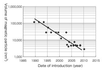
Fig. 3 Transition of the magnetic material volume
