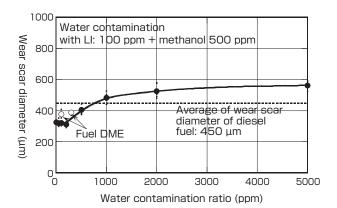
Fig. 7 Effect of water contamination on abrasion scar diameter<sup>[1]\*</sup> (water 0–5,000 ppm, methanol 500 ppm) \*Data added to ref. [1]
