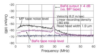
Fig. 11 Modulation spectra of the MP medium and the BaFe medium  $^{\scriptscriptstyle [10]}$
