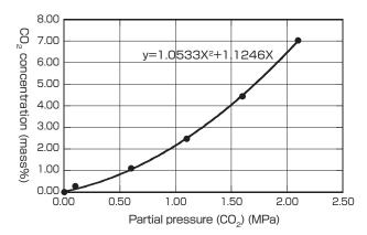
Fig. 14 Effect of  $CO_2$  partial pressure on  $CO_2$  solubility in DME<sup>[9]</sup>
