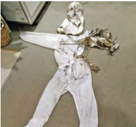
Damage caused by the dust explosion
