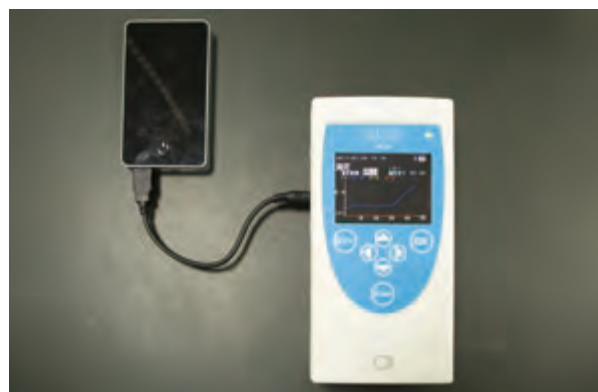
The developed mobile pathogen tester (the device on the left is a battery for a smartphone)
