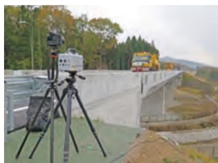
Setup for verification testing with digital Moiré technology
