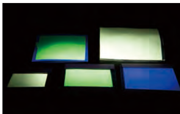
High-intensity phosphor films produced by the Photo MOD process
