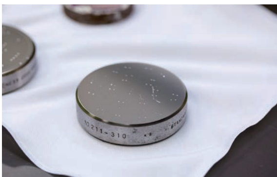
Measuring hardness by the depths of indentations
