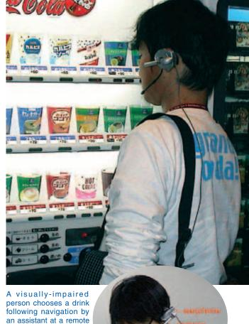
person chooses a drink following navigation by an assistant at a remote site, using an ear-phone type wearable camera system (with video camera, microphone and earphone).
