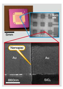
Figure 1. A chip integrated with 800 nanogap electrodes and its SEM photograph magnifying a nanogap part (molecule-sized gaps are constructed)
