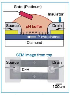
Figure 1. Schematic diagram of diamond pH sensor and SEM image
