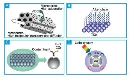
Figure. Enhancing photocatalyst performance through three-dimensional structure control A: Utilization of micro-mesopore silica adsorbent
