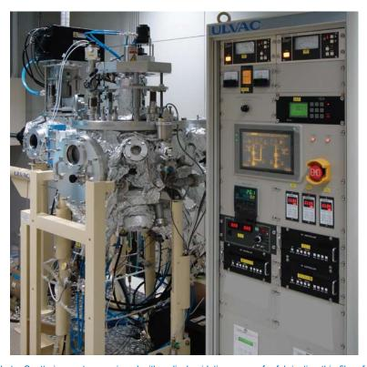
Photo. Sputtering system equipped with radical oxidation source for fabricating thin film of a transition metal oxide (the function of transition metal oxides changes largely depending upon the oxidation state, thus establishment of the thin-film deposition know-how is essential in the development of memory)
