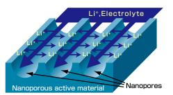
Figure 1. Image of diffusion path of lithium ions  $({\rm Li}^{\scriptscriptstyle \uparrow})$  through nanopores of a nanoporous active material
