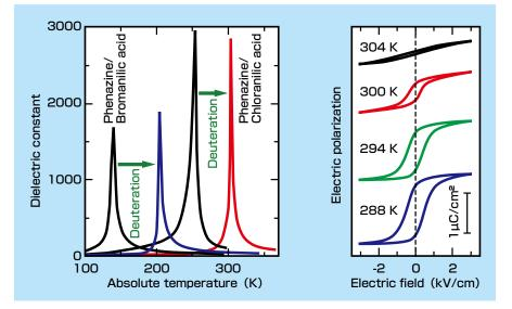
Figure 2. Dielectric property of a new organic ferroelectric material in which 2 species of  $\pi$ -electron molecules are bounded by strong hydrogen bonding
