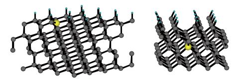
Figure 3. Optimized structure of phosphorous impurity atom (yellow) in surface region of hydrogenated diamond, Left: (111) surface, Right: (001) surface
