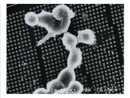
Figure 1. Method for preparation of nanopillar sheet using nanoimprinting technology (left) and electron microscope photograph of HeLa cells cultured upon nanopillars (diameter 0.5 µm) (right)
