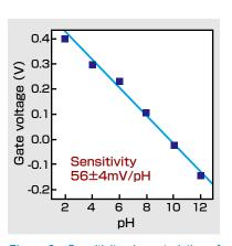
Figure 2. Sensitivity characteristics of diamond pH sensor
