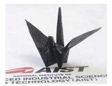
Photo 1. A folded-paper crane made using a high quality SWNT sheet
