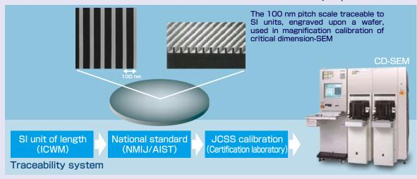
Figure. The 100 nm pitch nanoscale and the traceability system
