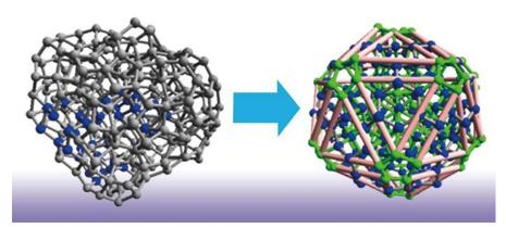
Figure 2. Simulation results of formation of a silicon regular icosahedral cluster
