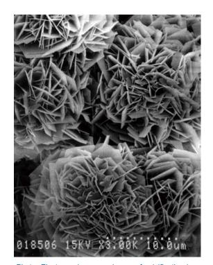
Photo. Electron microscope image of calcification by a phosphophoryn applied on agarose beads (Robust growth of apatite crystal was observed)
