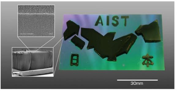
Photo 2. Carbon nanotubes which 'sustain Japan' (map of Japan made using vertically arranged SWNTs)
