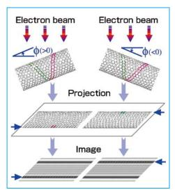
Figure 2. Discrimination of clockwise/anticlockwise winding of carbon nanotubes by sample tilting method
