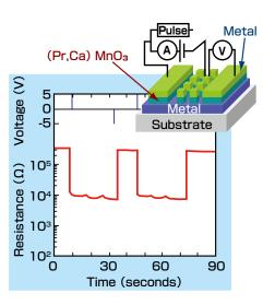
Figure 1. Colossal electro-resistance (CER) memory effect of perovskite manganese oxide
