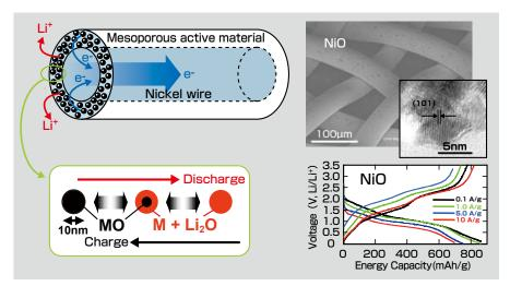
Figure 2. Achievement of both an electron conduction path and an ion diffusion path by structuring nanoporous active material on metal wire
