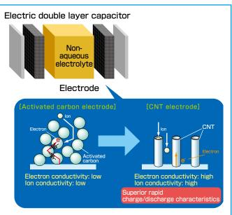
Figure 2. Comparison of activated electrode and CNT electrode
