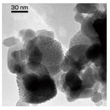
Photo. Palladium-supporting titanium oxide prepared by photodeposition
