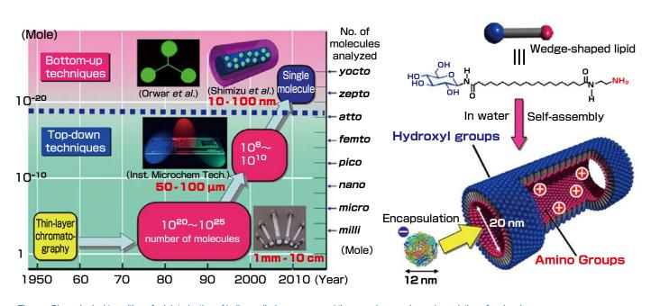
Figure. Chronological transition of miniaturization of hollow cylinder spaces, and the organic nanochannel consisting of molecules
