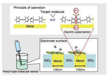
Figure 2. Electrode modification and principle of operation of pencil-type molecular sensor used in solution (when the target molecule was captured by the organic molecule adsorbed on the nanoelectrode surface, electric polarization is induced on the surface, and this change is detected)
