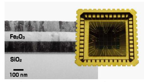
Figure 1. Cross sectional transmission electron microscope image of resistance random access memory structure consisting of iron oxide (left), and the prototype memory device of the same (right)
