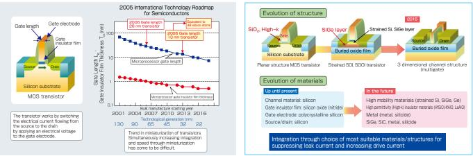
Figure 3 : Miniaturization towards a 10 nanometer gate length MOS transistor
