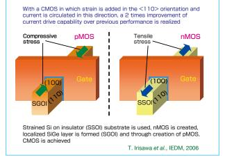
Figure 7: Most effective structure for uniaxial strained multigate CMOS (modulation of sub-band structure)
