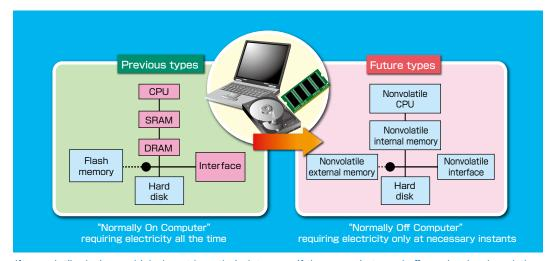
If nonvolatile devices, which do not lose their data even if the power is turned off, can be developed, then a great reduction in the electricity consumption of electronic data devices is expected.
