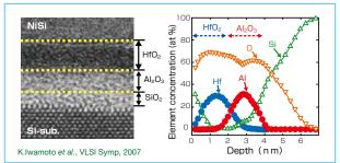
Figure 9: Cross-sectional transmission electron microscope photograph of high-k gate insulator film consisting of a gate stack comprised of 2 layers:  $HfO_2/Al_2O_3$  (left), and profile of composition of  $HfO_2/Al_2O_3/SiO_2$  layers by depth
