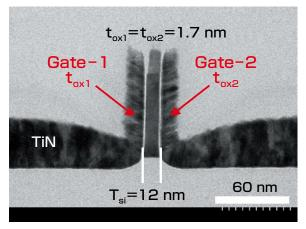
Figure 1: Prototype 4-terminal double-gate MOSFET (4T-XMOSFET)
