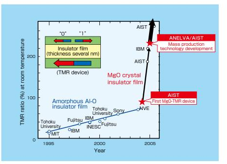
History of the performance improvements of tunnel magnetoresistance (TMR) devices which convert magnetic data to electric data AIST created a new type of TMR device which uses MgO as the insulator film.
