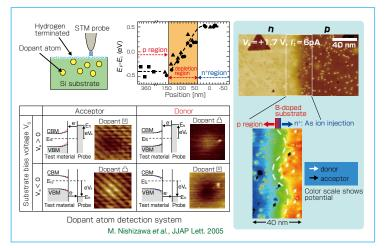
Figure 8 : Detection of individual impurity atoms in a Si crystal and simultaneous potential measurement by STM
