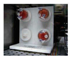
Figure 3: RWV (Rotating Wall Vessel) bioreactor
