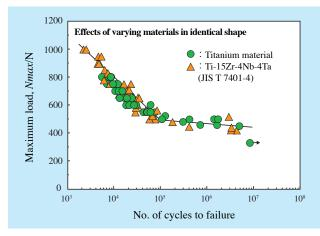
Figure 2: Results of 4-point bend test on straight plates
