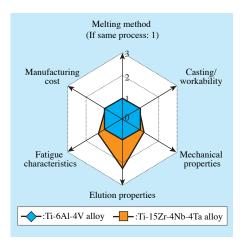
Figure 4: Comparison of titanium alloys
