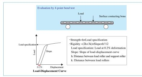
Figure 1: Method for mechanical properties evaluation of bone plate Types of bone plates include straight, angled, end, and others which are used bended, while the materials used are commercially pure titanium, titanium alloys, and stainless steel.
