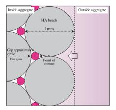
Figure 2: Pattern diagram of HA beads of 1 mm diameter at the closest packing structure
