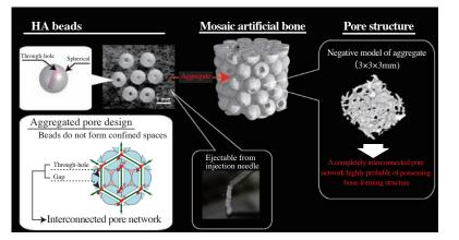
Figure 1: Mosaic artificial bone made using spherical artificial bone units (HA beads) HA beads can be aggregated into any arbitrary shape, upon which they form a completely interconnected pore network. The 1 mm  $\phi$  HA beads can be ejected from a 16G injection needle. The image of the HA bead aggregate is a 3D-CG model based upon microfocus X-ray CT data.
