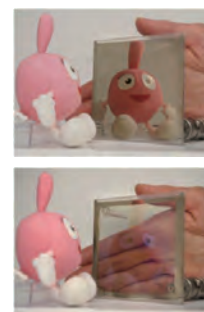
A newly developed switchable mirror coated with antireflection layer
