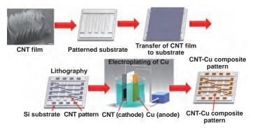
Fabrication protocol of the CNT-Cu composite
