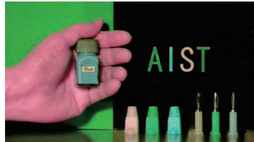
Example of images of objects taken in darkness by using the newly developed infrared color night-vision camera
