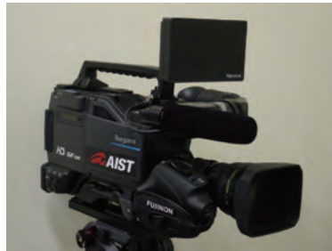
The newly developed HD infrared color night-vision camera
