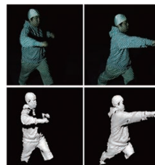
Measuring a person in motion by projecting wave grid pattern
