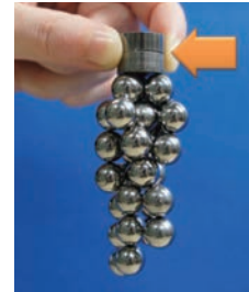
Developed Sm-Fe-N sintered magnet without heavy rare earth High-performance magnets attract 40 of 4-g iron balls.
