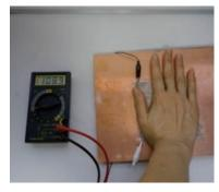
A flexible thermoelectric conversion film fabricated by using a printing process (left) and its electrical power-generation ability (right)
