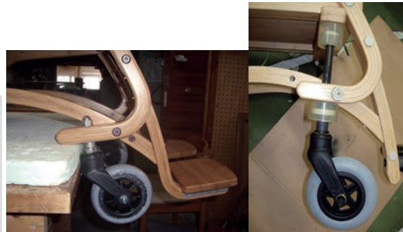
One-point support system (left) and two-point support system (right) of the frame
