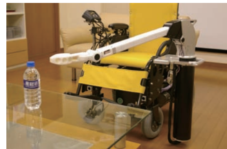
RAPUDA attached to an electric wheelchair
