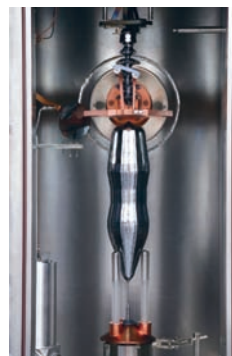
5 kg of ^{28}\text{Si} crystal (left) with enrichment factor of 99.99 % grown with float-zone (FZ) method, and laser interferometer (right) which measures the diameter of 1 kg of silicon sphere made from this crystal. Measurement of the diameter of the sphere is done with nanometer precision in a vacuum of strictly-controlled temperature by radiation shield.
