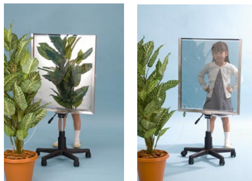
Large-size mirror switchable between reflective state (left) and transparent state (right).
