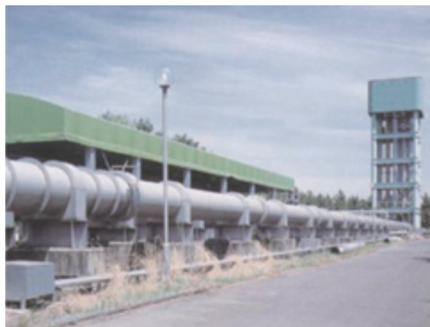
Figure 1: Overhead flow tank and test channels at ambient temperature.
