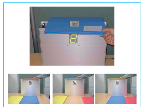
Figure 2: Demonstration of object identification using all-screen-printed RF ID tags on flexible plastic substrates.
