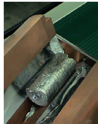
Photo: 5 mas % class Ca based Laves phase hydrogen adsorbing alloy prepared by the new melting method.
