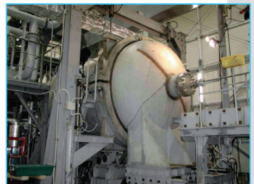
Photo. Sealed detonation chamber used to dispose of munitions.
