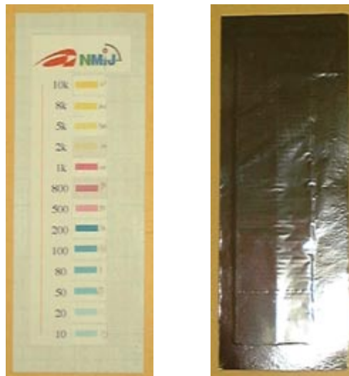
A printed radioactivity log scale. A broad range of radioactive concentrations can be obtained by setting inks, with different radioactive concentrations, in an inkjet printer and using the adjustment function of printing concentrations for each ink color.
