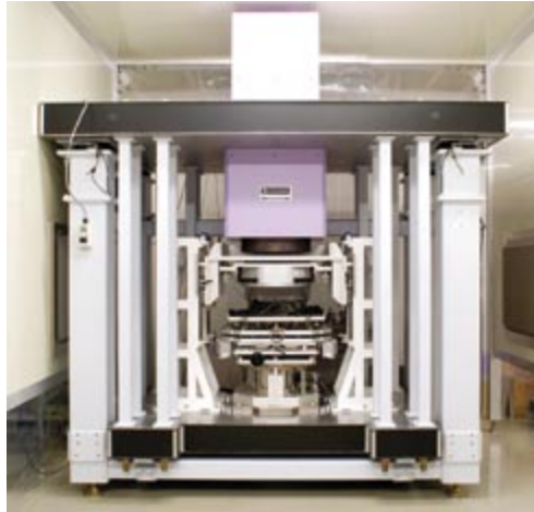
Flatness interferometer (measuring size: 300 mm diameter, uncertainty: 10 nm)
