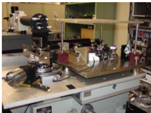
Photograph of the autocollimator calibration system consisting of the angle generator and angle interferometer.
