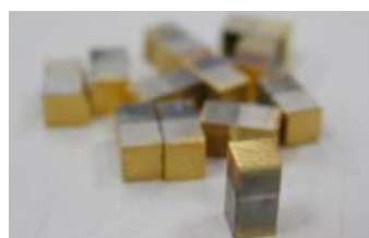
A picture of two stage segmented thermoelements prepared by not pressing
