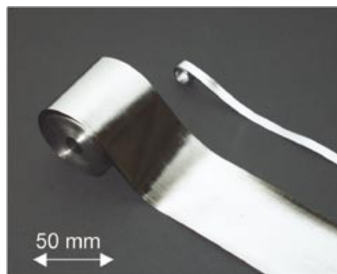
Amorphous alloy membranes quenched from the melt by courtesy of MITSUBISHI MATERIALS CO.
