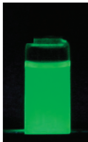
Photoluminescence from water-soluble ZnS/CdSe nanocrystals prepared by a Microfluidic reactor
