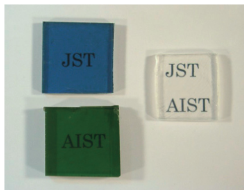
Waste colored glass (left) and porous transparent colorless glass obtained from the waste glass (right)
