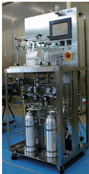
Practical device for the automated manufacture of hyperpolarized xenon gas developed through the AIST research
