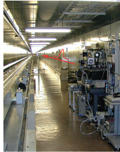
Femtosecond-Comb Distance Meter in the optical testing tunnel at AIST. The arrow in the photograph indicates the laser beam.
